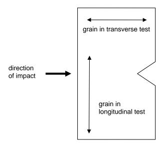
When the directional force of the hit goes across the grain (as it does in a "longitudinal" test), it is harder to fracture the specimen than if the force goes parallel to the grain. It takes more energy to break the steel across the grain. That is why a longitudinal specimen has higher notch toughness than a transverse specimen. In other words, it will take more foot pounds (or joules) of absorbed energy to break a longitudinal specimen.
