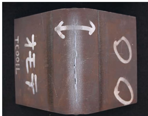
Example of crack which occurred during bending
