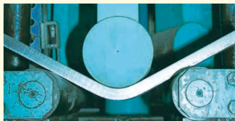
Geometry of bending test piece (JIS Z 2248)
