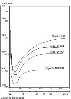
Measured at midthickness, 3/8" (9.5mm) min thickness
