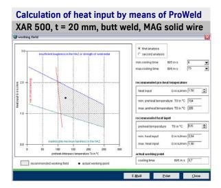
During welding it has to be assured that the cooling times are in the recommended range by using suitable welding conditions taking into account the necessary preheating temperature. Joining with lower-alloyed steels is generally not problematic if welding conditions are adapted to the XAR® steel. Assistance in choosing appropriate welding conditions is also offered by our computer programme ProWeld. General recommendations on arc welding are given in EN 1011- part 1 and part 2.
