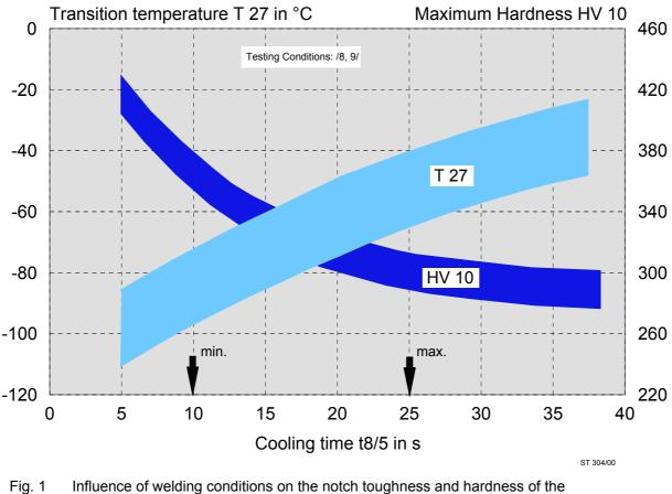
Fig. 1 Influence of welding conditions on the notch toughness and hardness of t affected zone of N-A-XTRA<sup>®</sup> multilayer welds
