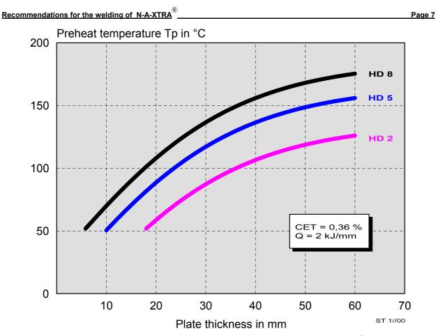
Fig. 2 Preheat temperature and interpass temperature for welding N-A-XTRA<sup>®</sup>-steels
