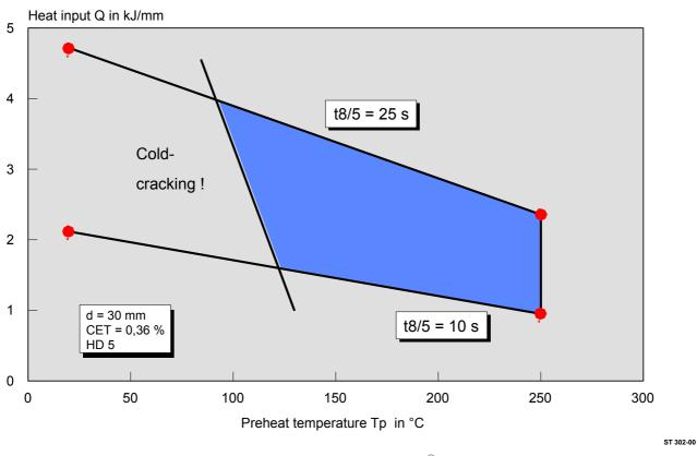
Fig. 3 Favoured field of welding conditions for N-A-XTRA<sup>®</sup> - steels on the basis of: - minimum transition temperature  $T_{27} = -40$  °C - maximum hardness in the HAZ = 380 HV 10
