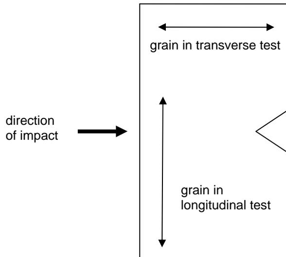
When the directional force of the hit goes across the grain (as it does in a “longitudinal” test), it is harder to fracture the specimen than if the force goes parallel to the grain. It takes more energy to break the steel across the grain. That is why a longitudinal specimen has higher notch toughness than a transverse specimen. In other words, it will take more foot pounds (or joules) of absorbed energy to break a longitudinal specimen.
