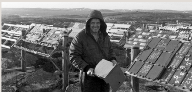
The primer performance to resist corrosion is continuously tested at our test site, located on an island on the Swedish west coast.
